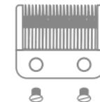
(1) The end of the upper blade teeth should be 0.5 to 1 mm behind the lower blade holes. This is important so that the razor does not cut too close or allow the moving blade to touch the skin.
